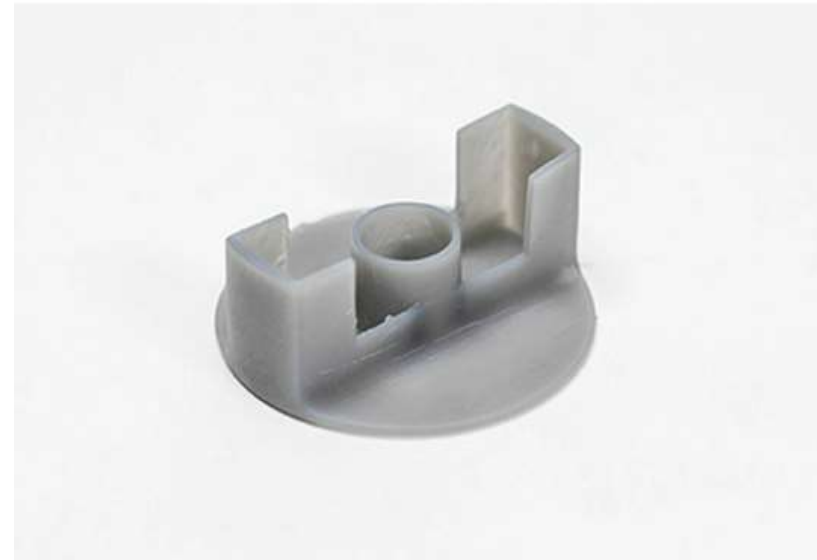
The finished shaft end cap with support structures removed
