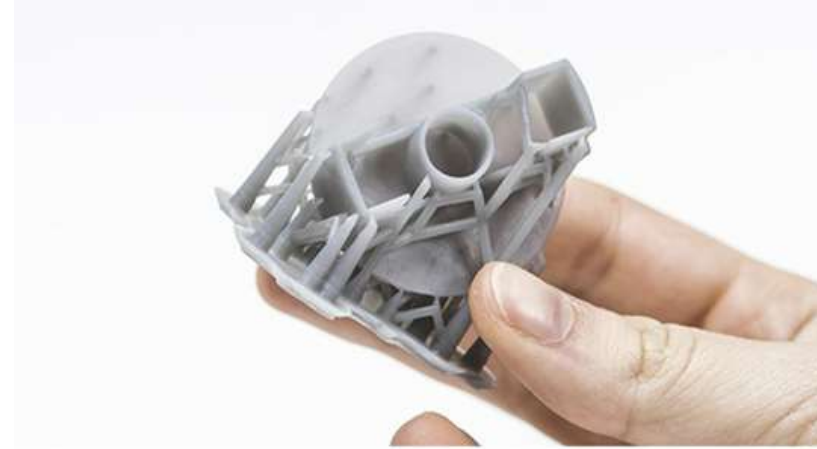
The shaft end cap after being removed from the build platform with support structures still attached
